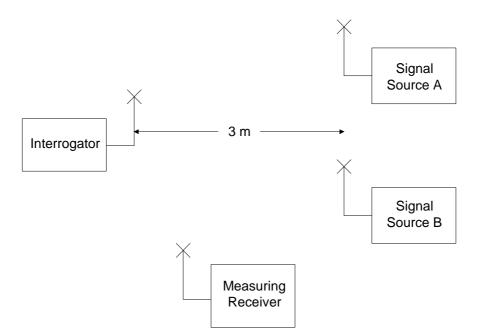
Figure B.4: Radiated measurement of blocking
