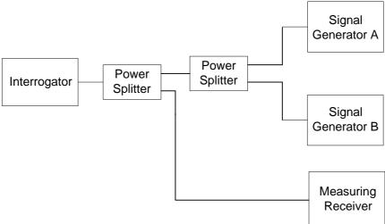
Figure B.5: Conducted measurement of blocking
