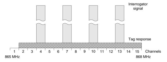
Figure 1: Diagram of channel plan
