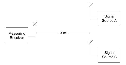
Figure B.3: Calibration of field levels
