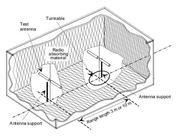
Figure A.1: A typical anechoic chamber
