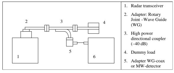
Figure D.1: Measurement of the operation frequency and the pulse power
