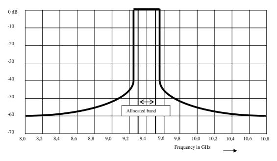
Figure D.3: Maximum permitted out-of-band-emissions power level
