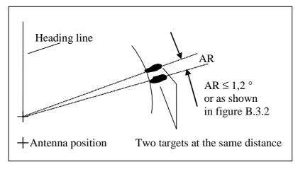
Figure C.3: Definition of the Azimuthal Resolution (AR)
