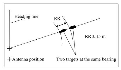
Figure C.2: Definition of the Radial Resolution (RR)
