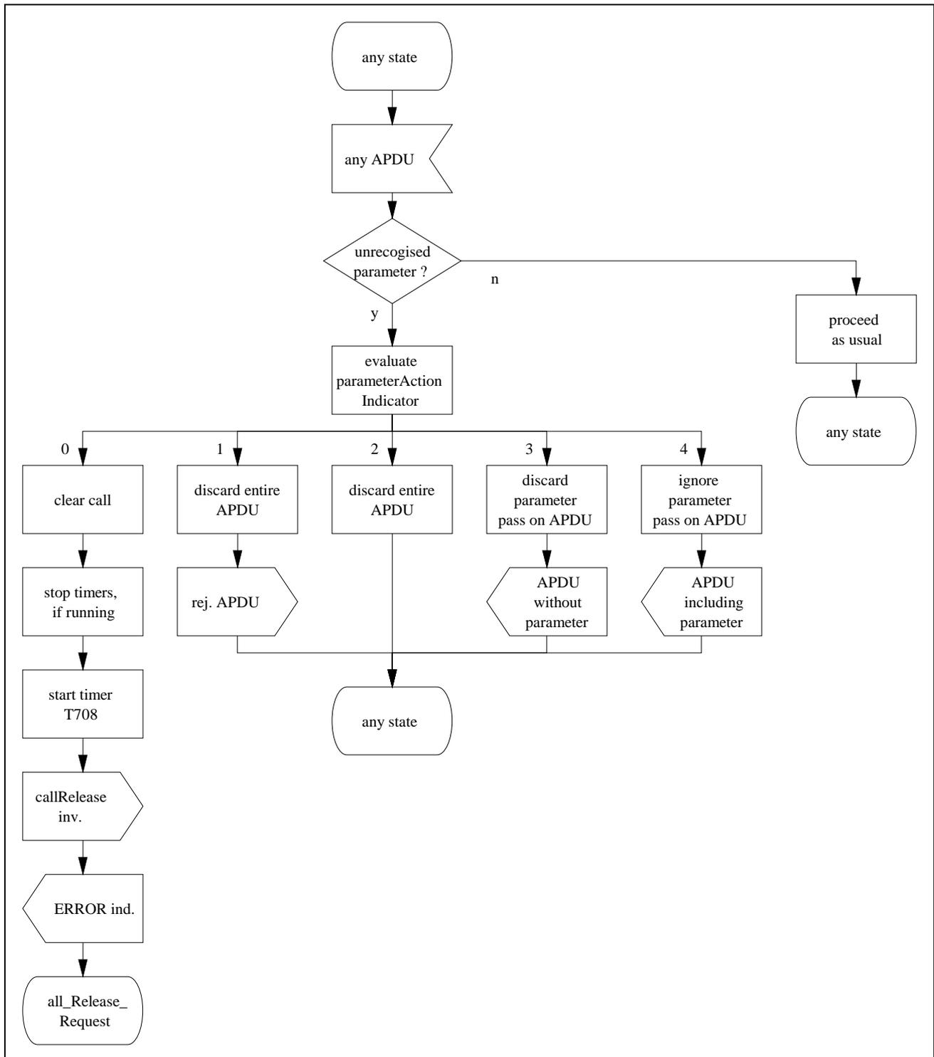
Figure 29: SDL for the handling of unrecognised parameters within CC operations
