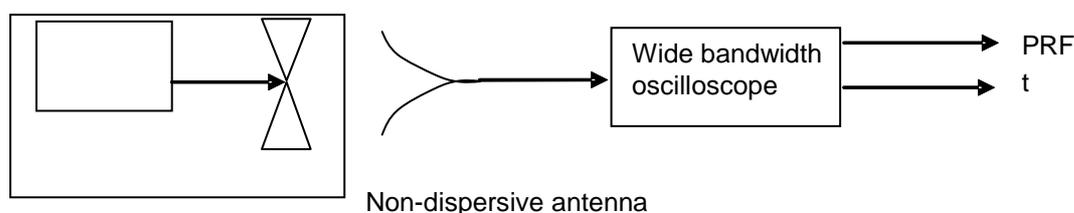
Figure D.1: Test setup 1
