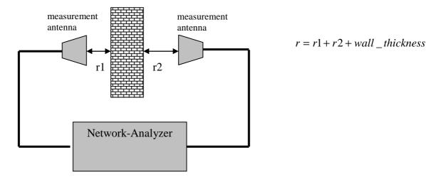
Figure D.2: Attenuation measurement, example: wall
