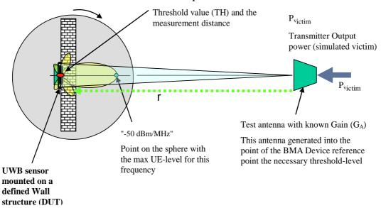
Figure 7: Test set-up for LBT function, example: Building Material sensor
