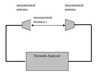
Figure D.1: Calibration setup
