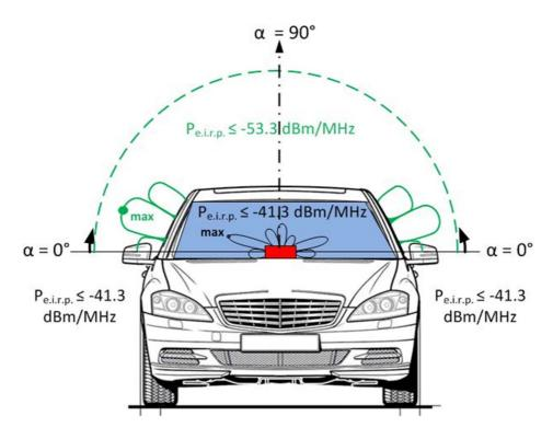
NOTE: The exterior limit refers to the maximum mean spectral density e.i.r.p. measured outside the vehicle and every local maximum should be below the limits.
