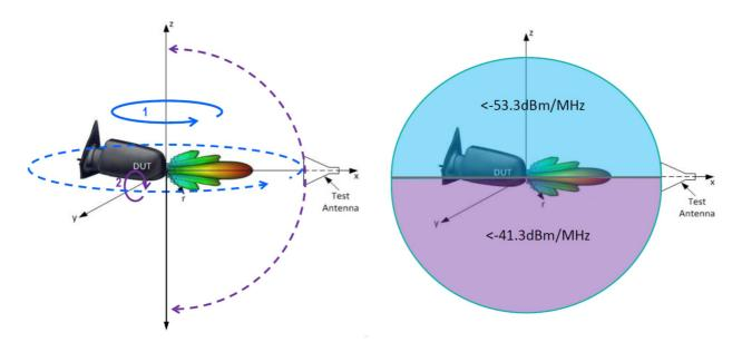
Figure D.2: Full spherical scan of a mirror
