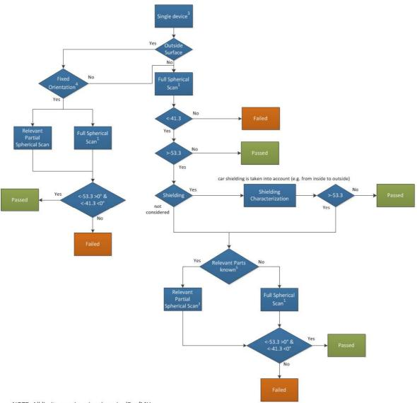
NOTE: All limits are given in e.i.r.p. in dBm/MHz
