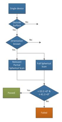
Figure C.1: Measurement Flow
