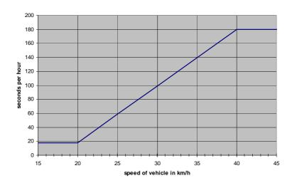
Figure 2: Long term duty cycle: Sum of transmitter on time with respect to speed of the vehicle (ECC/DEC(06)04 [i.11])
