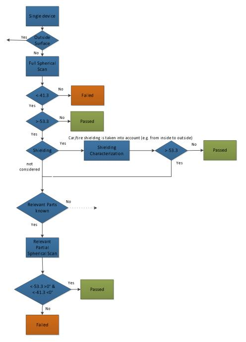
Figure D.1: Measurement Flow (DUT)
