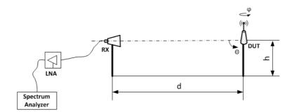
Figure 2: Spherical scan setup with rotation and tilt of the DUT
