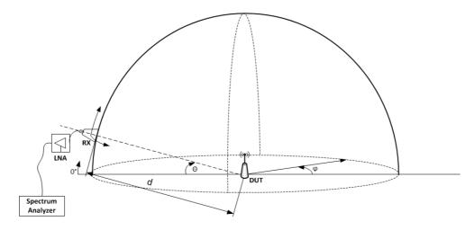
Figure 1: Spherical scan setup using automatic test antenna placement
