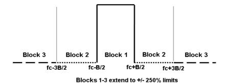
Figure 1: Measurement Mask normalized to channel bandwidth
