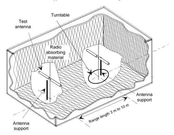
Figure C.1: A typical anechoic chamber
