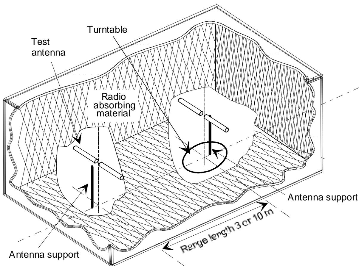
Figure A.1: A typical Anechoic Chamber
