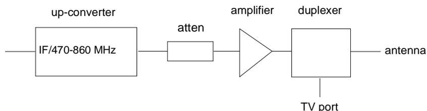
**Figure 63: RF stage Block Diagram**
