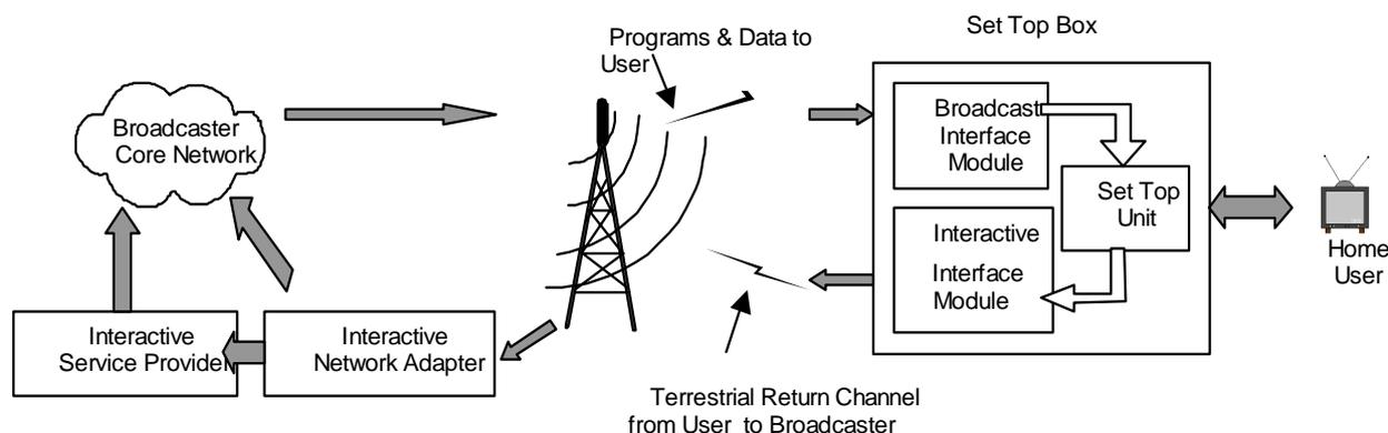
**Figure 4: Illustration of the DVB-RCT network**
