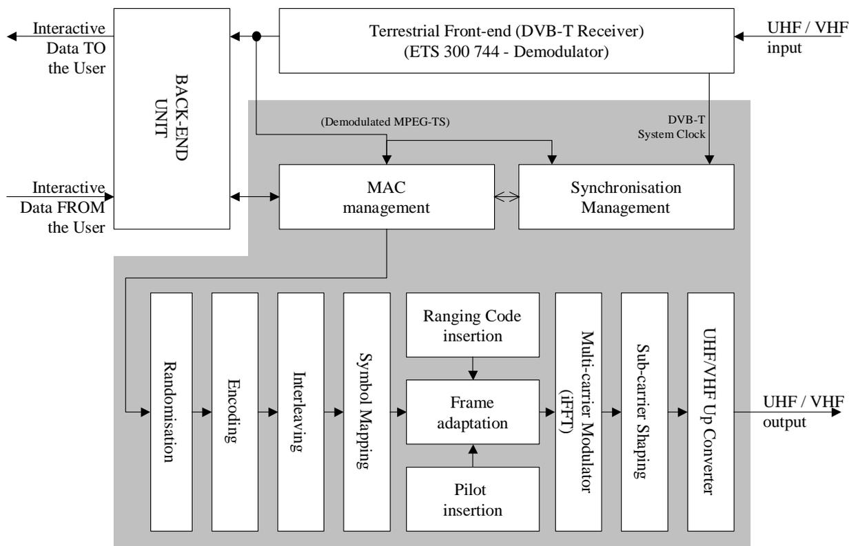
**Figure 5: Conceptual Block Diagram for the DVB-RCT**
