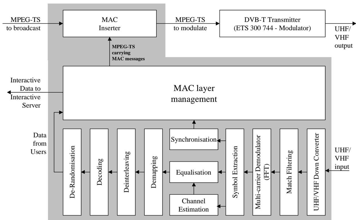
**Figure 6: Conceptual Block Diagram for the Base Station**
