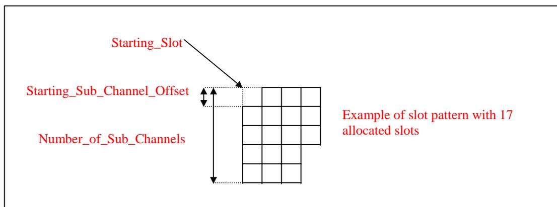
Figure 49: Slot Pattern Structure
