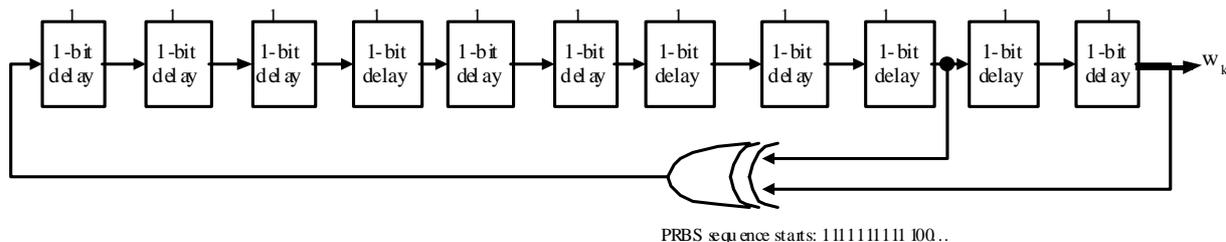
**Figure 20: PRBS sequence generator for Pilot modulation**
