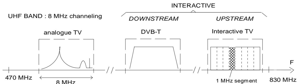
Figure 54: Sharing of Return Channel spectrum within UHF Broadcasting Bands
