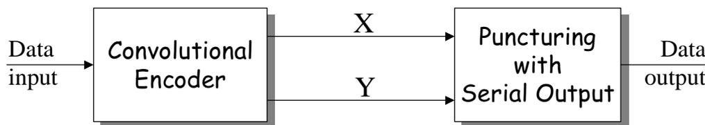
Figure 16: Convolutional encoder Block diagram
