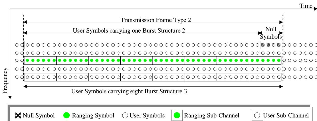
**Figure 10: Organization of TF2 frame structure (time domain)**
