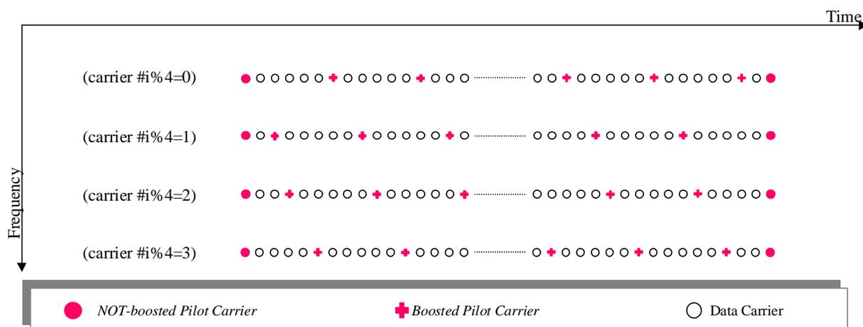
**Figure 22: Pilot insertion scheme for the BS1 mini-bursts**
