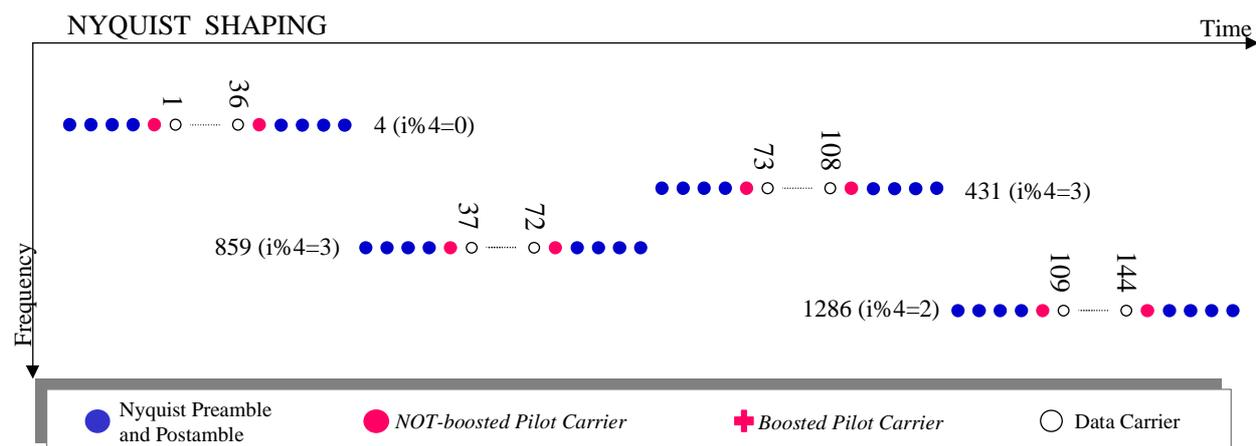
Figure 26: BS1 with frequency hopping and Nyquist shaping
