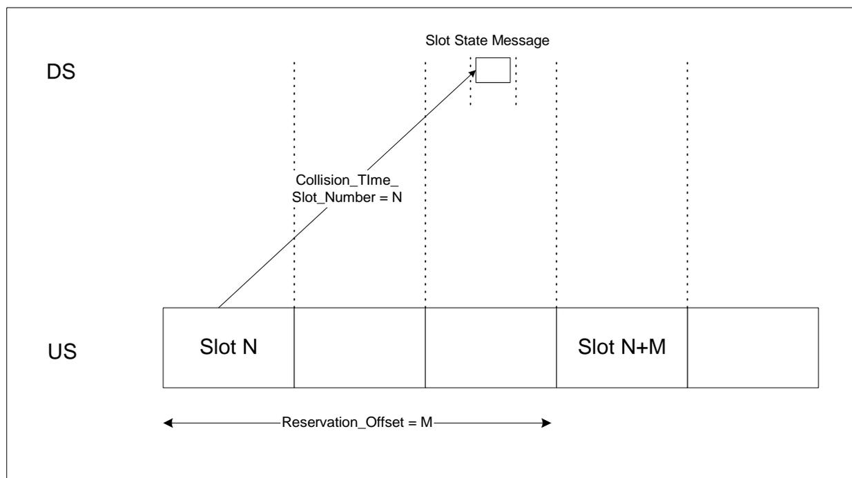
Figure 47: Examples of configurable Slot\_State message delay
