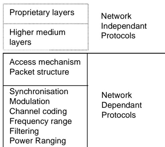
**Figure 1: Layer structure for generic system reference model**
