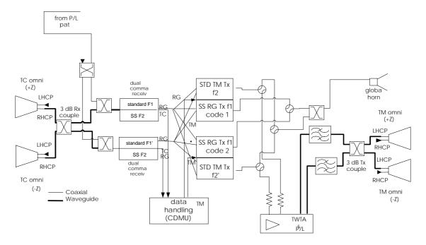
Figure A.4: Configuration 3 typical TCR/RF architecture
