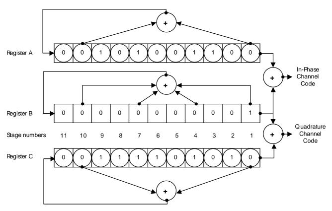
Figure E.5: Examples of register loading for gold codes based on code set 1 (circled positions can be programmed by the user)
