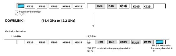
Figure A.1: Typical TCR frequency plan (Ku-Band)
