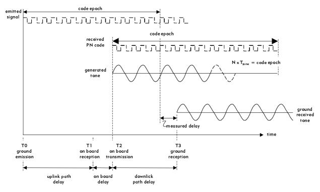
Figure B.2: RG hybrid timing diagram
