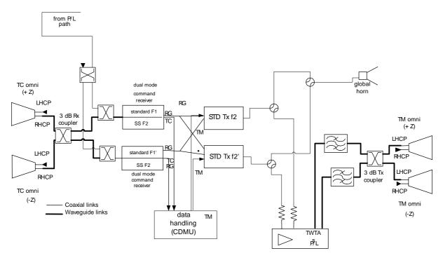
Figure A.3: Configuration 2 typical TCR/RF architecture
