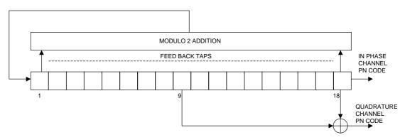
Figure E.3: Telemetry downlink and ranging PN code generator
