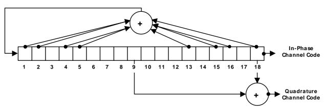
Figure E.6: Examples of tap connections for maximum length codes based on code set 1
