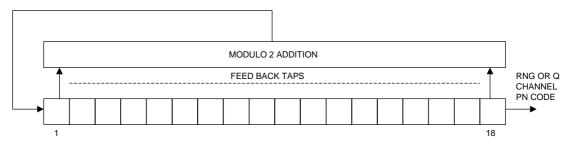
Figure E.2: Ranging uplink or quadrature channel PN code generation
