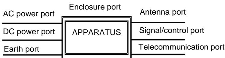
**Figure 1: EUT Ports for EMC purposes**
