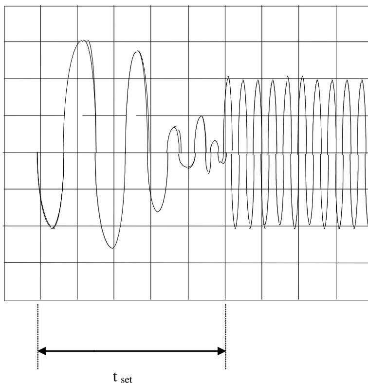
**Figure 6: Modulator attack time, typical oscilloscope trace**
