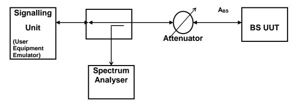
Figure 5.4.2.1-1: Test Setup for BS transmitter adjacent channel leakage ratio measurement
