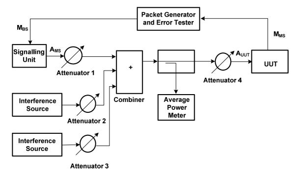
Figure 5.4.9.1-1: Test setup for receiver intermodulation response test
