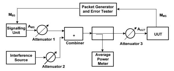
Figure 5.4.8.1-1: Test Setup for BS receiver blocking measurement
