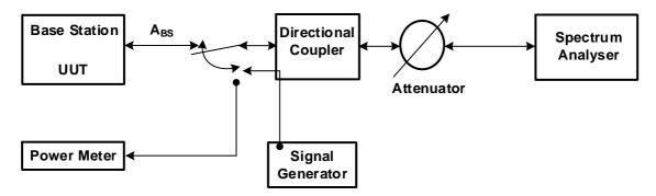
Figure 5.4.5.1-1: Test Setup for transmit intermodulation measurement
