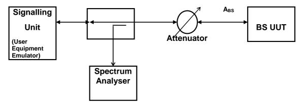
Figure 5.4.1.1-1: Test Setup for BS transmitter spectrum emission mask measurement
