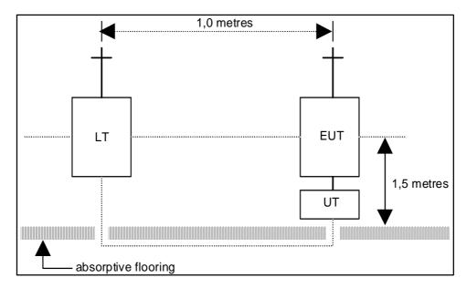
Figure 20: Testing arrangement
