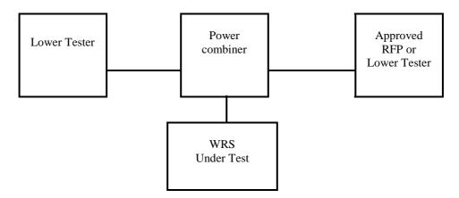
Figure 3: WRS testing as an RFP
