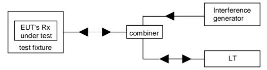
Figure 13: Measuring arrangement for calibration
