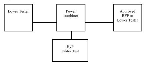
Figure 43: HyP testing as an RFP
