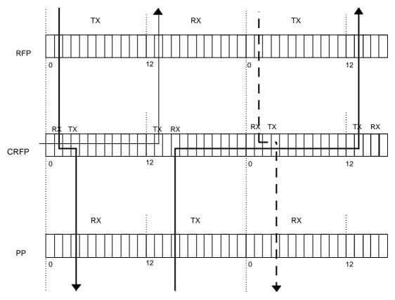
Figure 4: Typical frame multiplexing structure of the CRFP
