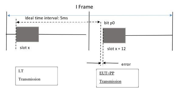
Figure 30: PP packet transmission error definition
