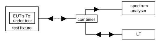
Figure 12: Measuring arrangement for calibration
