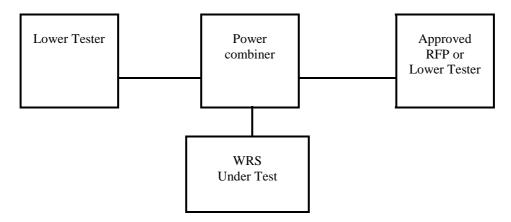
Figure 41: WRS testing as an RFP
