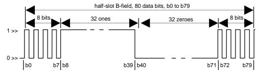
NOTE: Bits  $b_0$  to  $b_7$  and  $b_{72}$  to  $b_{79}$  are alternating 1 s and 0 s with the even order bits  $(b_0, b_2, b_4,...)$  set to "1" and the odd-order bits  $(b_1, b_3, b_5,...)$  set to "0".
