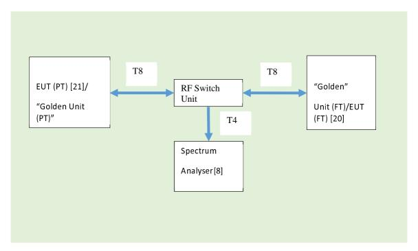
Figure 39: Channel Release Test Setup
