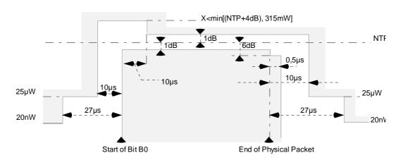
Figure 1: Physical packet power-time template
