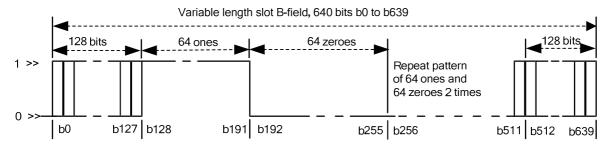
NOTE: Bits  $b_0$  to  $b_{127}$  and  $b_{512}$  to  $b_{639}$  are alternating 1 s and 0 s.
