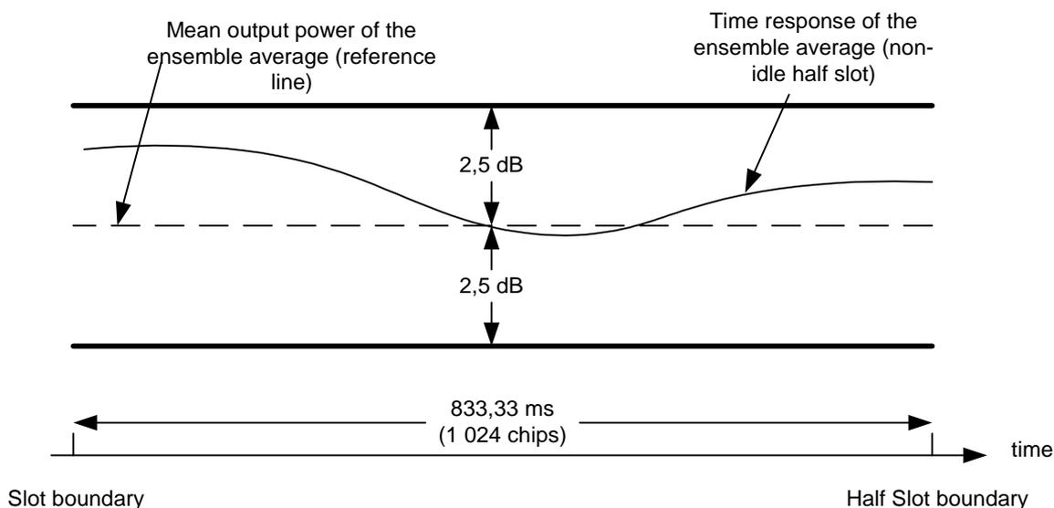
**Figure 1: Transmission envelope mask (average non-idle half slot)**
