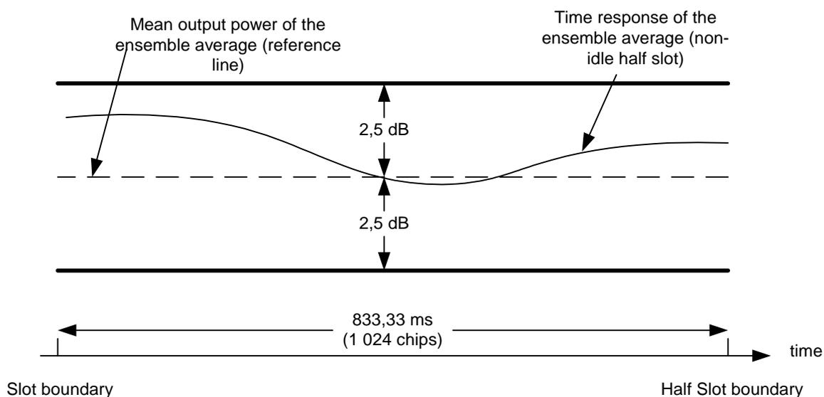
**Figure 2: Transmission envelope mask (average non-idle half slot)**
