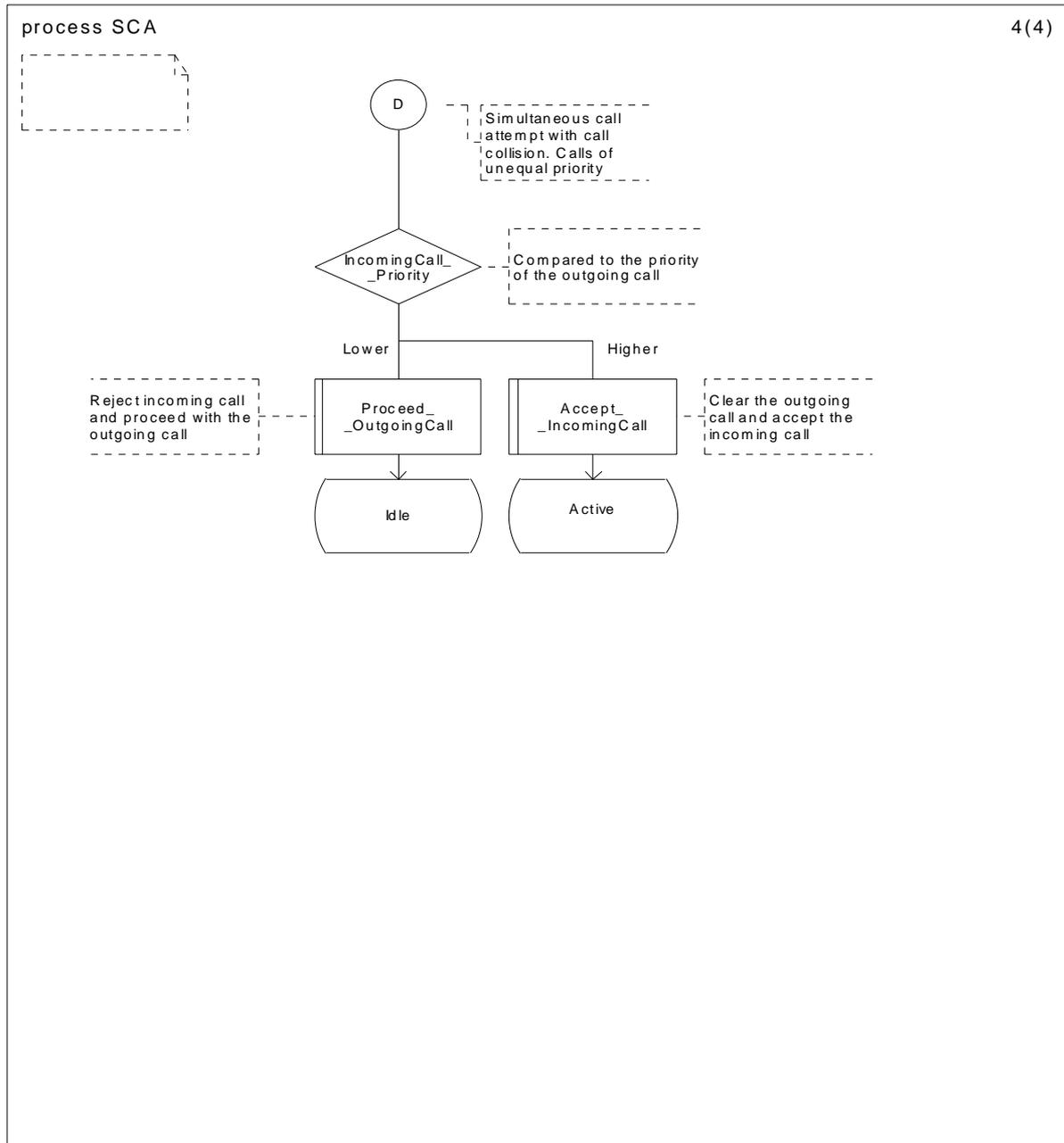
Figure C.1 (sheet 4 of 4): SDL for the detection and resolution of simultaneous call attempts
