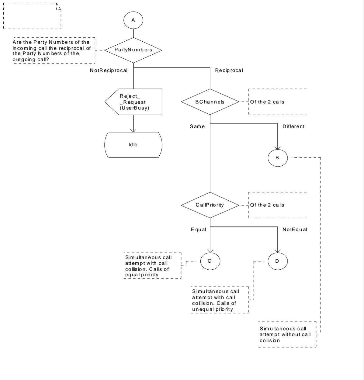
Figure C.1 (sheet 2 of 4): SDL for the detection and resolution of simultaneous call attempts
