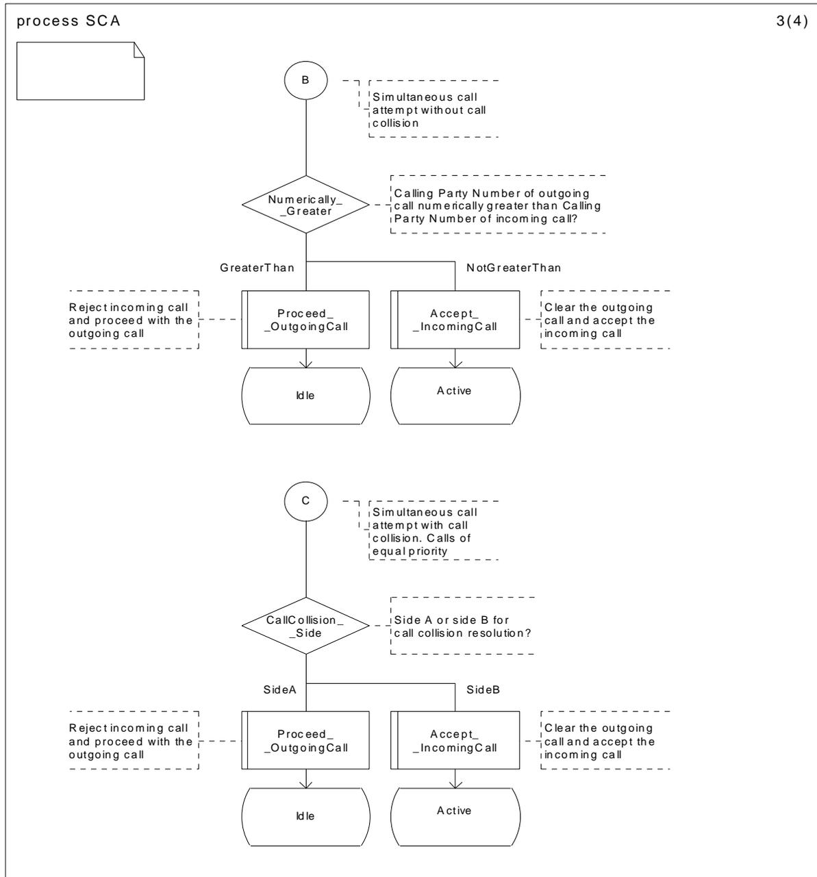
Figure C.1 (sheet 3 of 4): SDL for the detection and resolution of simultaneous call attempts
