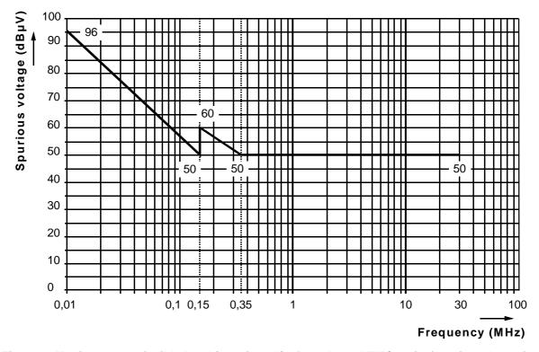
Figure 2: Maximum permissible level (quasi-peak) of conducted EMC emissions into the mains
