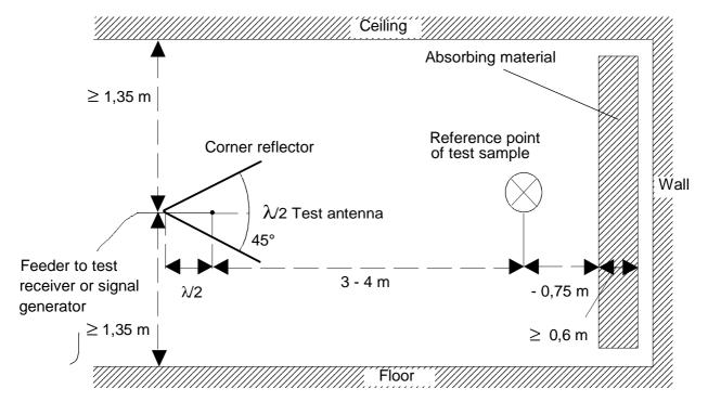
Figure B.3: Indoors site arrangement (shown for horizontal polarization)
