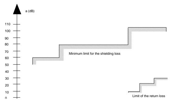
Figure B.4: Specification for shielding and reflections
