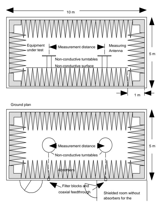
Figure B.5: Example of construction of an anechoic shielded chamber
