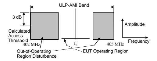
Figure 2: Spectrum Mask for Test of clauses 5.3.7.1.4.1 and 5.3.7.1.4.2
