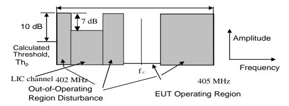
Figure 3: Spectrum Mask for Test of clause 5.3.7.1.6.1
