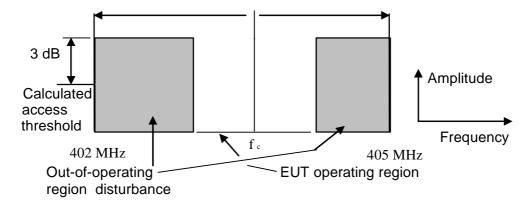
Figure 1: Spectrum Mask for Test of clauses 5.3.7.1.3.1 and 5.3.7.1.3.2
