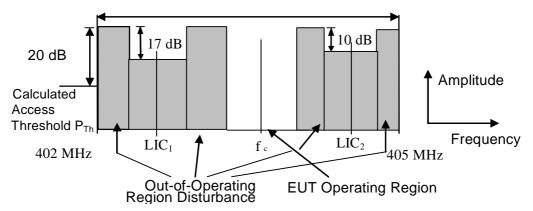
Figure 4: Spectrum Mask for Test of clause 5.3.7.1.8.1
