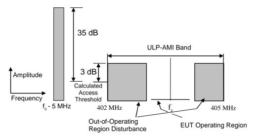
Figure 5b: Spectrum Mask for Test (fc - 5 MHz)of clause 5.3.8.1
