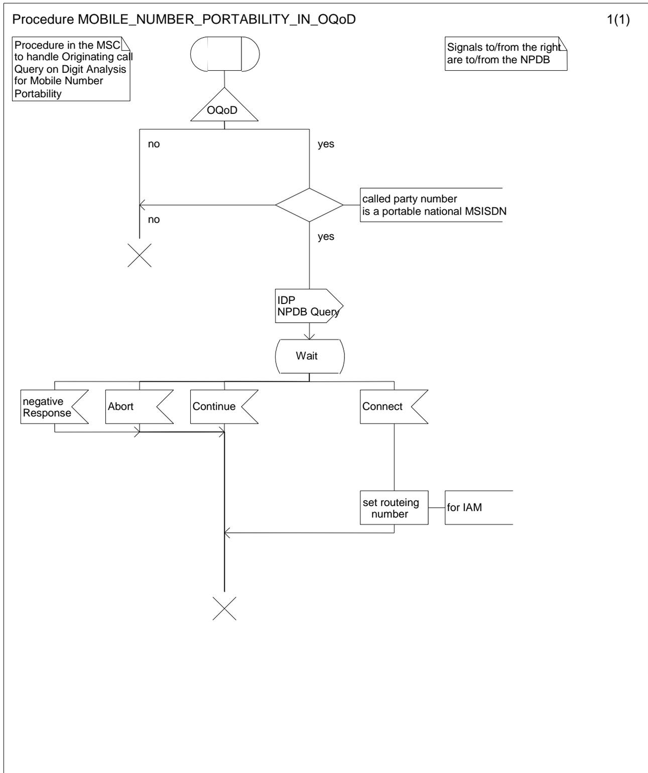
Figure A.3.3: Procedure MOBILE\_NUMBER\_PORTABILITY\_IN\_OQoD
