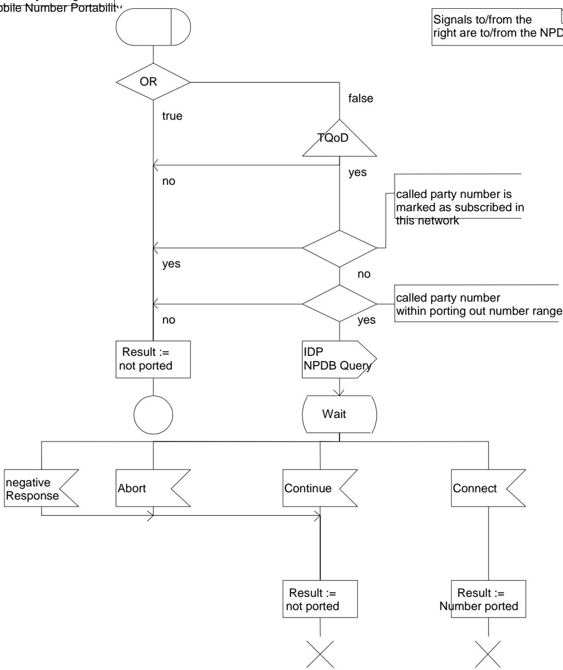
Figure A.3.2: Procedure MOBILE\_NUMBER\_PORTABILITY\_IN\_TQoD
