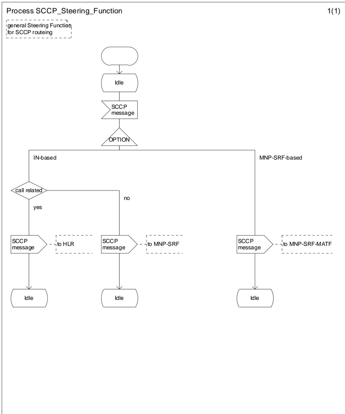
**Figure 1: Steering Function for SCCP Message routing**
