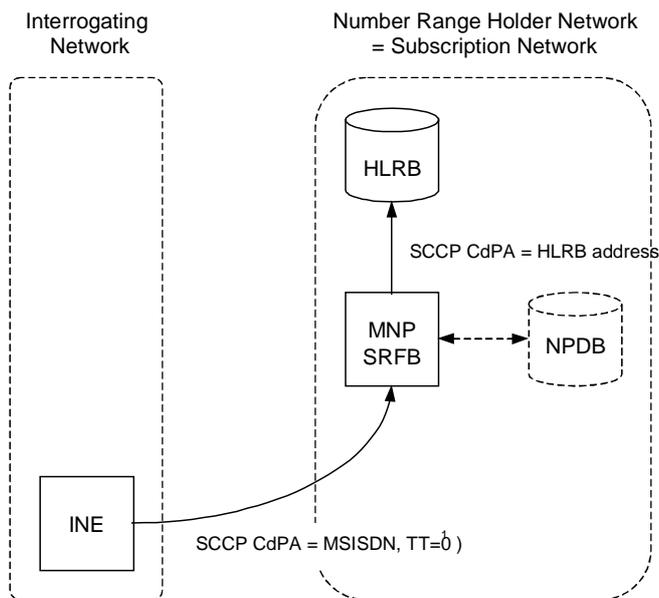
**Figure B.2.1: MNP-SRF operation for routeing a non-call related signalling message for a non-ported number where the interrogating network is inside the portability domain and indirect routeing is used or the interrogating network is outside the portability domain**
