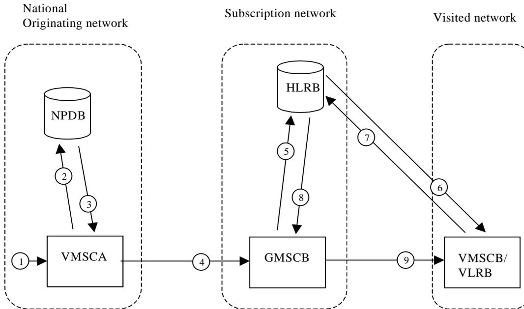
**Figure A.1.4.2: Call to a ported number using OQoD procedure**
