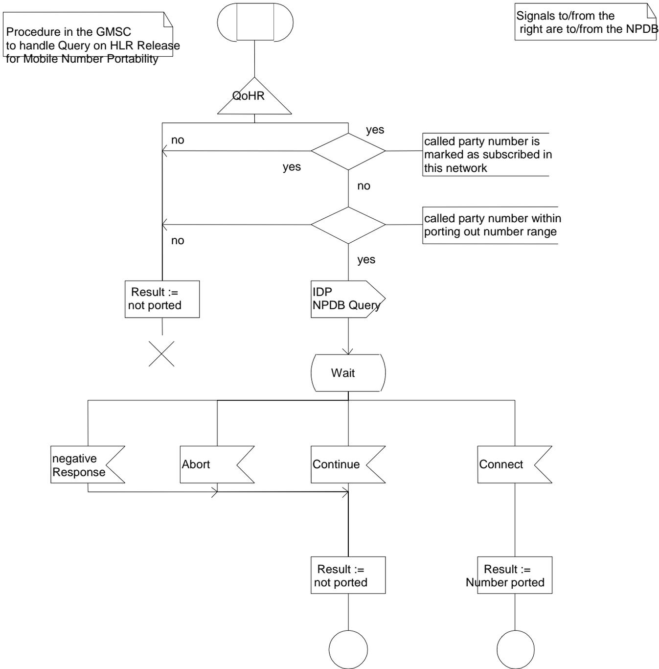
Figure A.3.1: Procedure MOBILE\_NUMBER\_PORTABILITY\_IN\_QoHR
