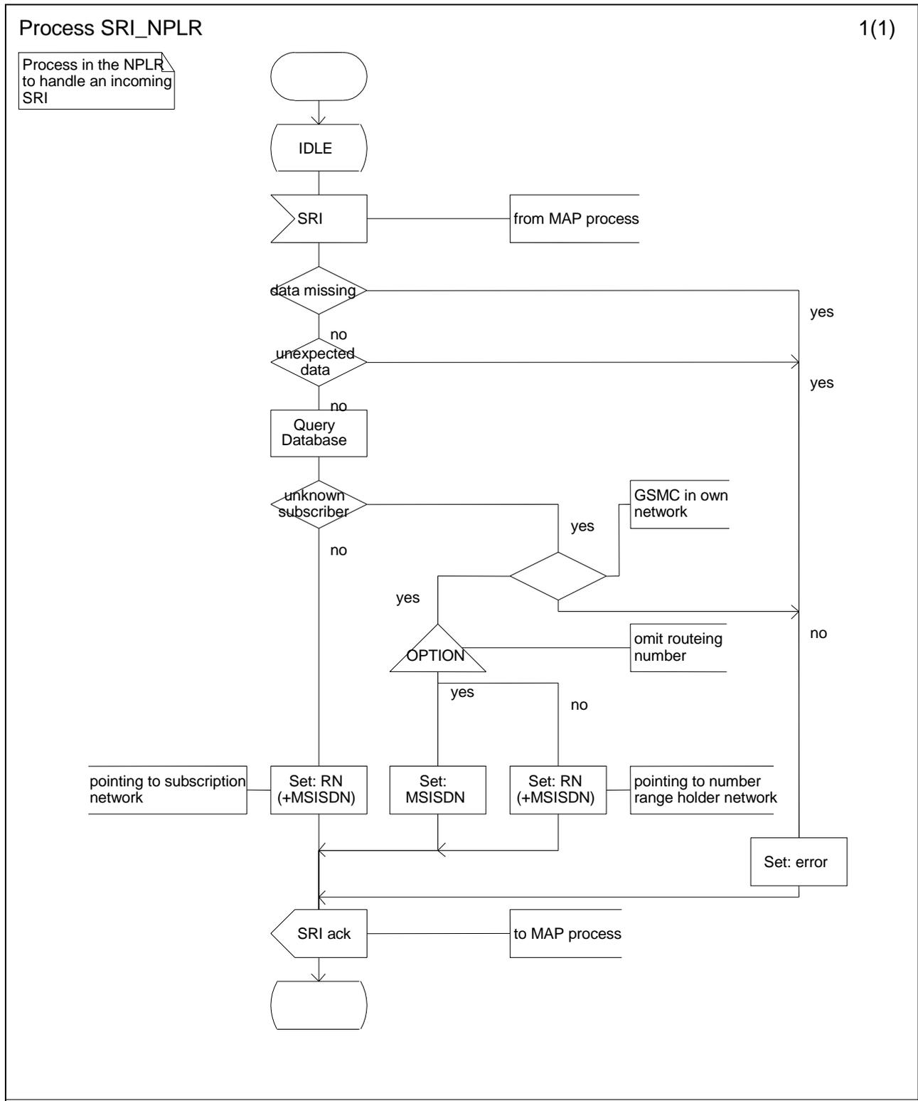
Figure C.2.2: Process SRI\_NPLR
