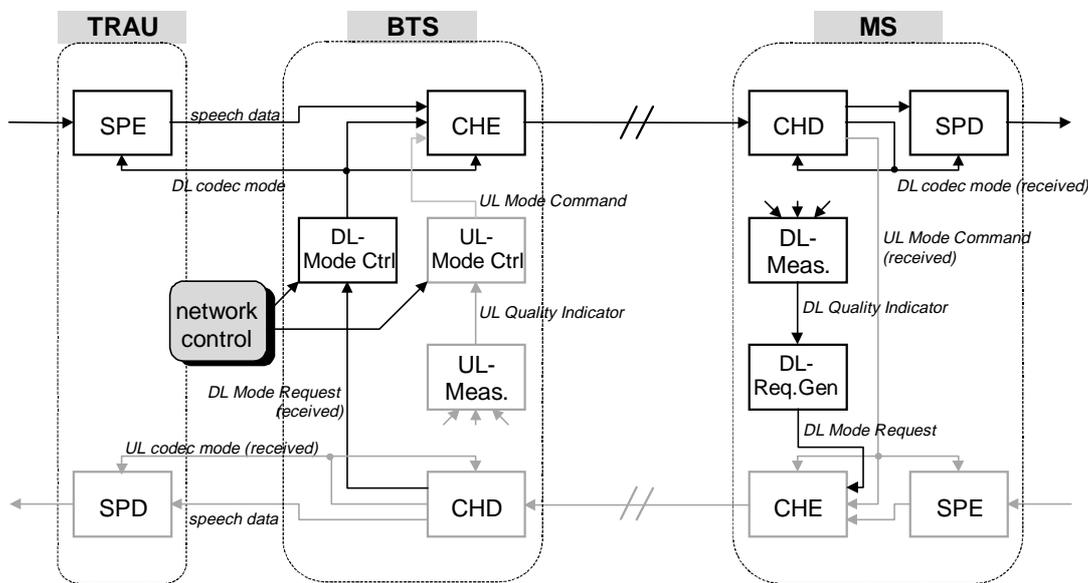
Figure 2: Block diagram of the AMR system.
