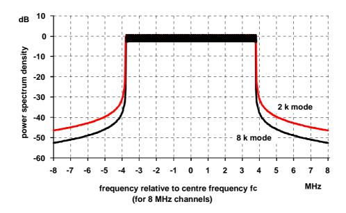
Figure 4: Theoretical UHF DVB transmission signal spectrum for guard interval  $\Delta = T_1/4$
