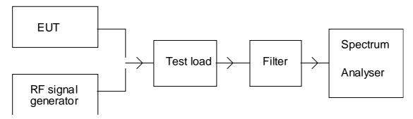
Figure 6: Measurement arrangement for conducted emissions
