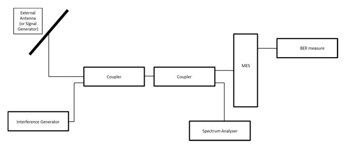
Figure 7: Measuring system set-up for Adjacent Channel Selectivity and Blocking Characteristics
