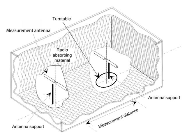
Figure B.3: A typical Fully Anechoic Room
