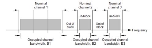
NOTE: Nominal channel bandwidths are 8 MHz and 24 MHz. The total nominal channel bandwidth is 40 MHz.
