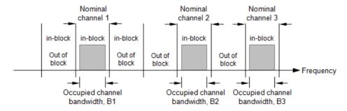
NOTE: Nominal channel bandwidth is 8 MHz. The total nominal channel bandwidth is 24 MHz.
