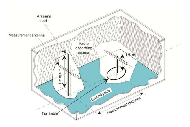
Figure B.2: A typical Semi Anechoic Room
