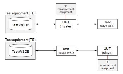
Figure 2: Test set up
