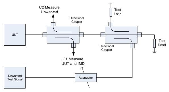
Figure 3: Transmitter Intermodulation Test Set-Up
