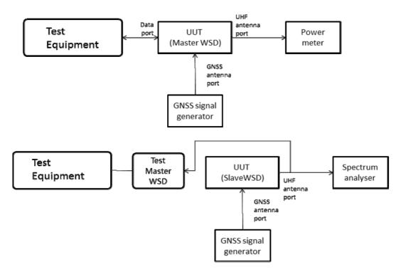
Figure 5: Test arrangement for Geo-location capability
