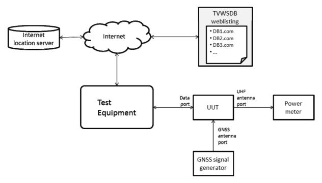
Figure 4: Test arrangement for database discovery and access
