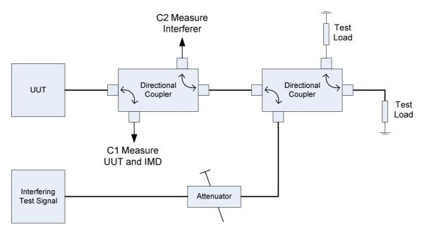
Figure 3: Transmitter Intermodulation Test Set-Up
