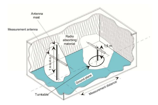
Figure B.2: A typical Semi Anechoic Room
