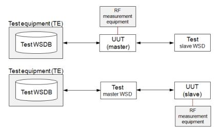
Figure 2: Test set up
