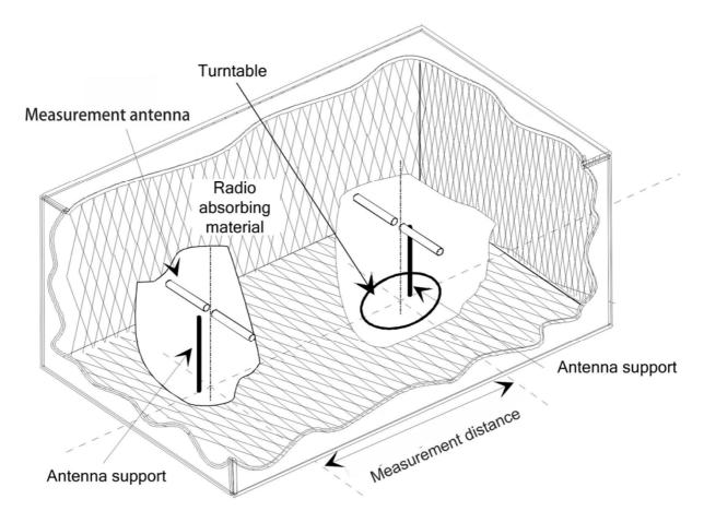
Figure B.3: A typical Fully Anechoic Room
