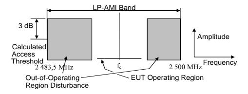
Figure 2: Spectrum Mask for Test of clauses 5.3.3.3.1 and 5.3.3.3.2
