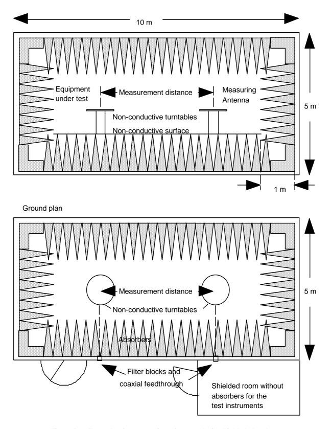
Figure B.6: Example of construction of an anechoic shielded chamber
