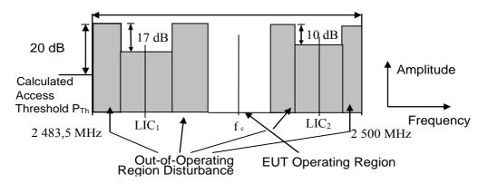
Figure 4: Spectrum Mask for Test
