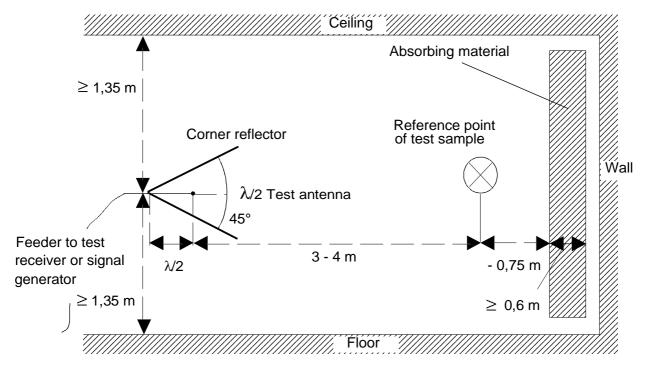
Figure B.4: Indoors site arrangement (shown for horizontal polarization)
