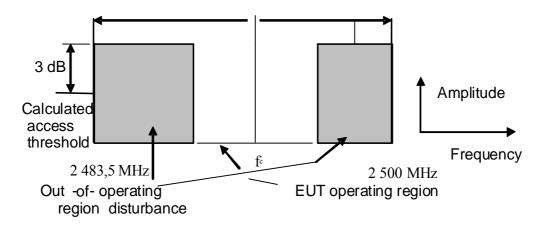
Figure 1: Spectrum Mask for Test of clauses 5.3.3.2.1, 5.3.3.2.2 and 5.3.3.2.3
