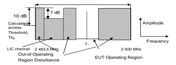
Figure 3: Spectrum Mask for Test
