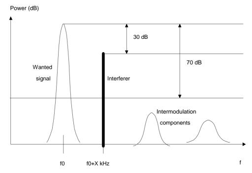
Figure 5.3.6-1: Example of TX intermodulation attenuation
