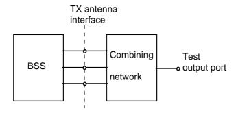
Figure B.2-2: Transmitter test setup
