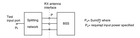
Figure B.2-1: Receiver test setup
