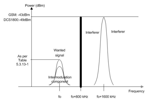
Figure 5.3.13-1: Example of RX intermodulation rejection
