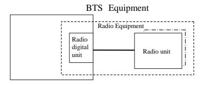
Figure 5.3.16-3: BTS with multiple enclosure solution
