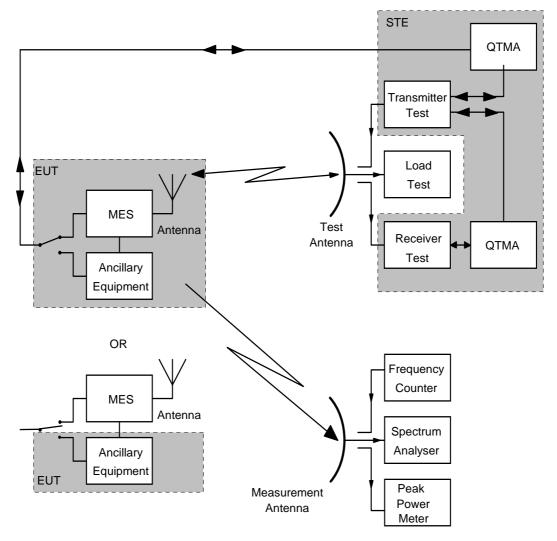
Figure 1: Suggested test configuration
