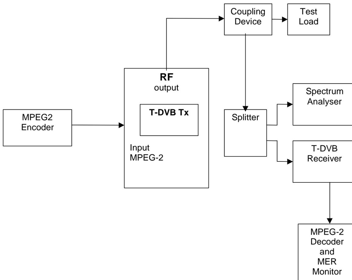
**Figure 2: Typical test arrangement for the performance assessment of a T-DVB transmitter, example**
