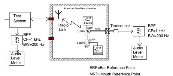
NOTE: The EUT is in position during calibration of the uplink, but not during calibration of the downlink.
