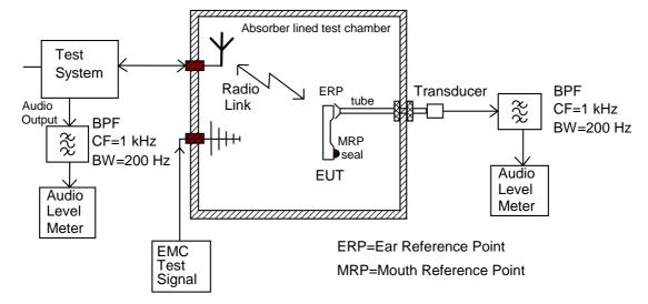
Figure 1: Audio breakthrough measurement, test set-up
