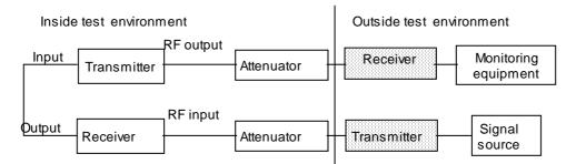
Figure 5: Test configuration of transceivers
