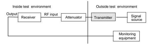
Figure 4: Test configuration for receivers
