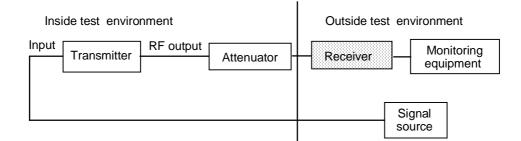
Figure 3: Test configuration for transmitters
