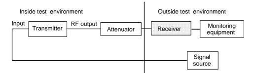
Figure 3: Test configuration for transmitters
