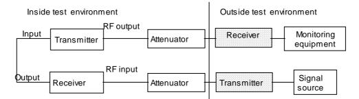
Figure 5: Test configuration of transceivers
