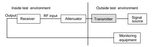
Figure 4: Test configuration for receivers
