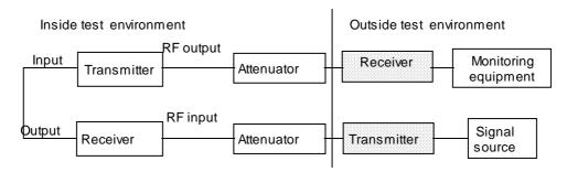
Figure 5: Test configuration of transceivers
