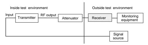
Figure 3: Test configuration for transmitters
