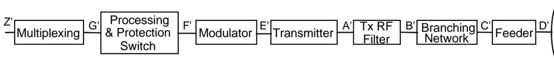
NOTE 1: For the purposes of defining the reference points, the branching network (B' to C') does not include a hybrid.
