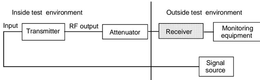
**Figure 3: Test configuration for transmitters**
