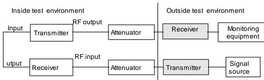
**Figure 5: Test configuration of transceivers**
