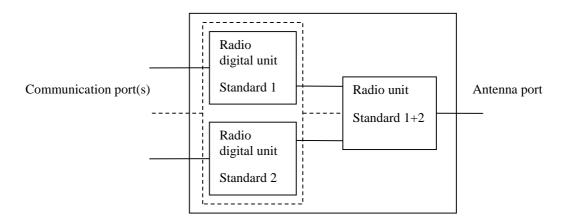
Figure 2: Multi-standard-radio equipment
