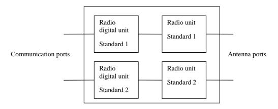
Figure 1: Multi-radio equipment
