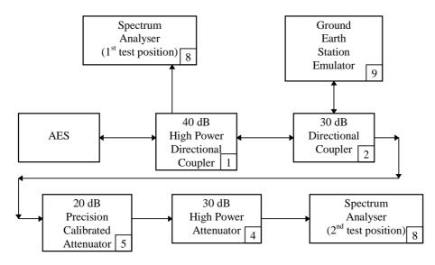
Figure C.2: Measurement arrangement for carrier-off
