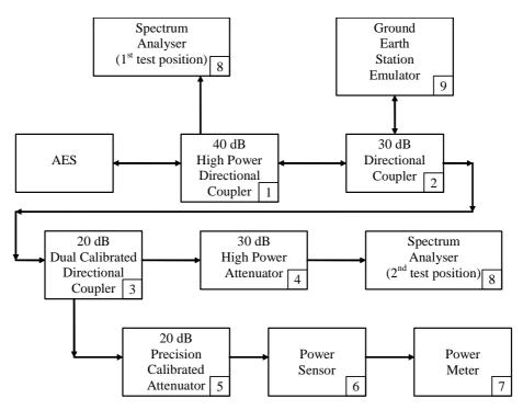
Figure C.1: Measurement arrangement for conducted emissions
