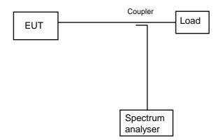
Figure 7: Test arrangement - transmit output power density measurement
