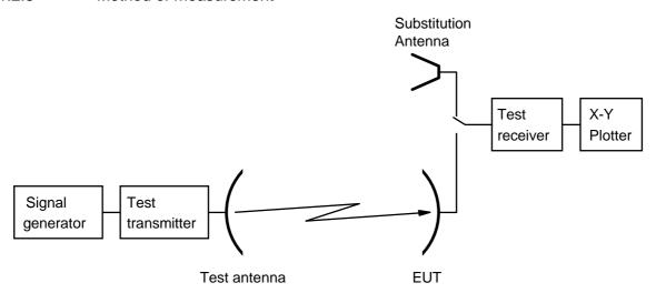
Figure 8: Test arrangement - antenna transmit gain measurement
