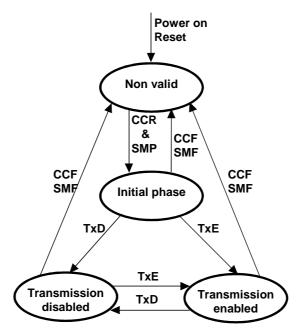
SMP: System Monitoring Pass; SMF: System Monitoring Fail;
