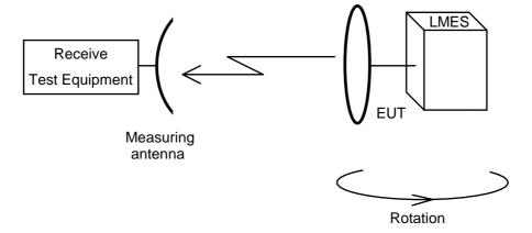
Figure 3: Test arrangement - emissions measurement, second axis
