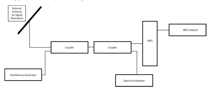
Figure 6: Measuring system set-up for Adjacent Channel Selectivity and Blocking Characteristics
