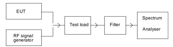
Figure 5: Measurement arrangement for conducted emissions
