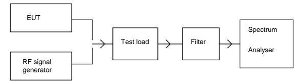
Figure 6: Measurement arrangement for conducted emissions
