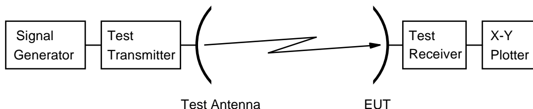
Figure 16: Test arrangement - antenna receive pattern measurement
