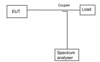
Figure 9: Test arrangement-transmit output power density measurement
