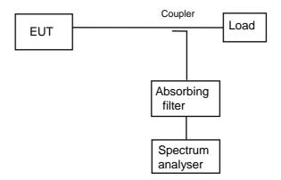
Figure 7: Test arrangement - on-axis spurious radiation measurements at the antenna flange
