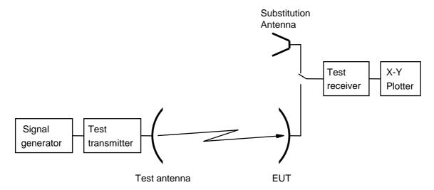
Figure 10: Test arrangement-antenna transmit gain measurement
