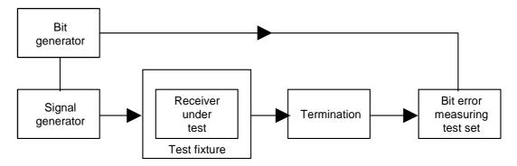
Figure B.2: Measurement arrangement No.2
