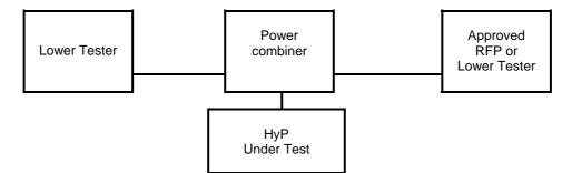
Figure 8: HyP testing as an RFP
