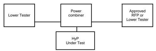
Figure 42: HyP testing as an RFP
