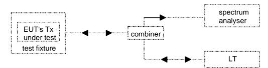
Figure 14: Measuring arrangement for calibration
