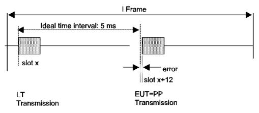
Figure 33: PP packet transmission error definition
