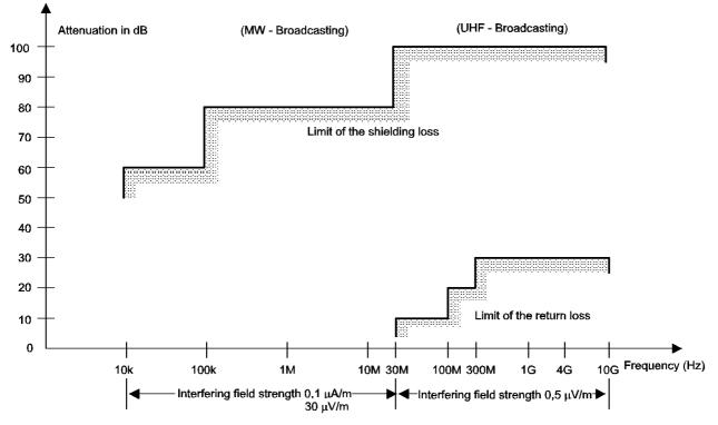
Figure 12: Shielding and wall return loss
