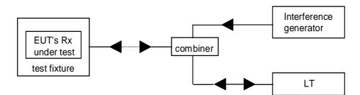
Figure 15: Measuring arrangement for calibration
