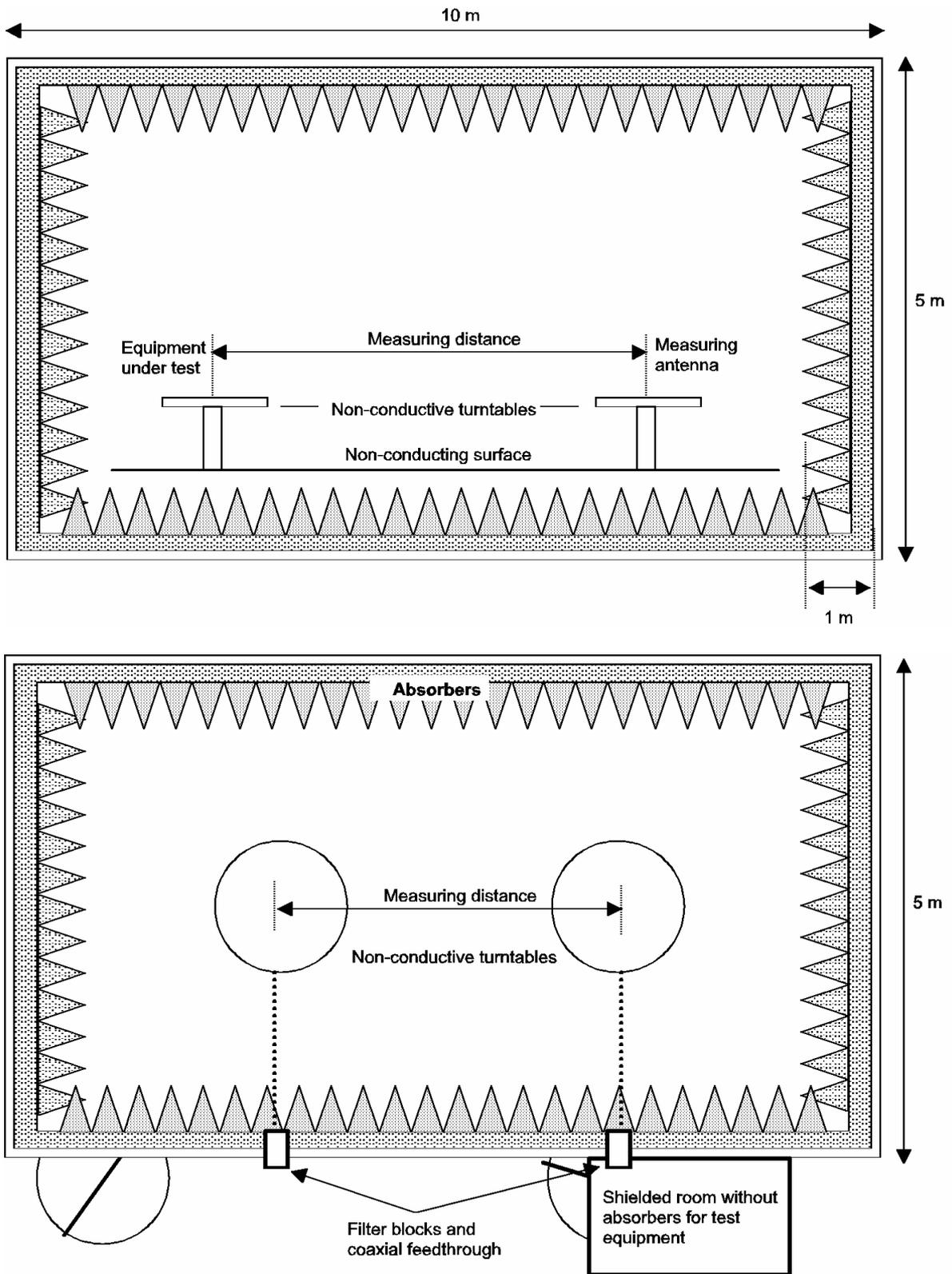
Figure 13: Construction example
