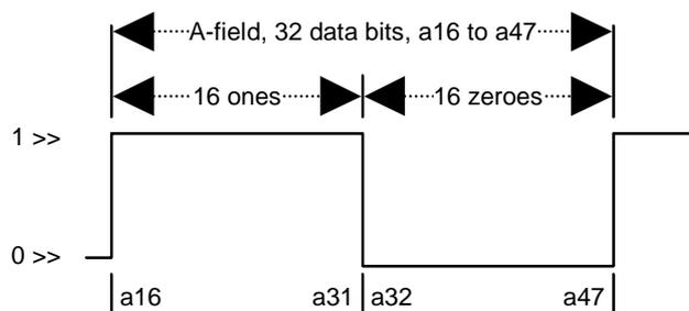
**Figure 35: Test packet structure for case 2, A-field**
