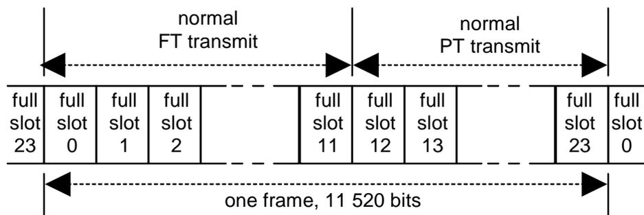
**Figure 2: Frame and full-slot structure**
