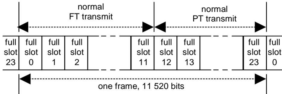
**Figure 2: Frame and full-slot structure**
