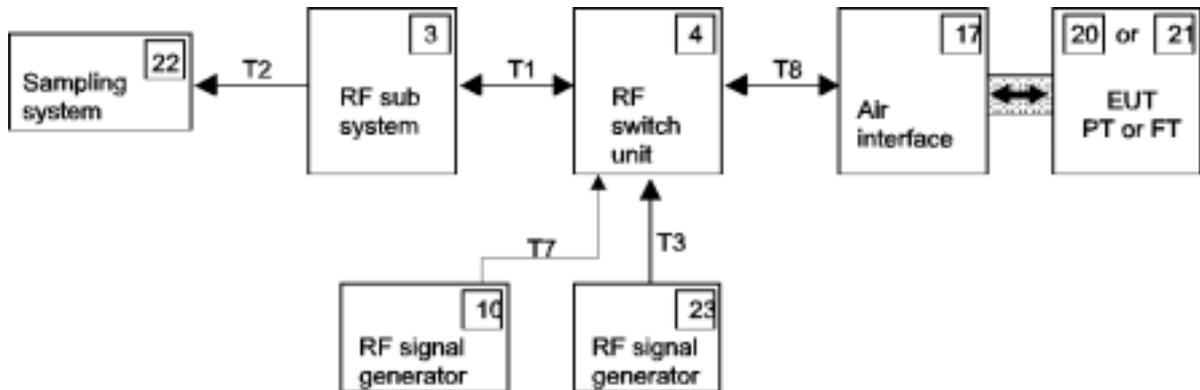
Figure 20: Test setup 3
