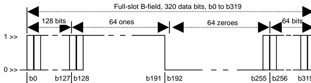
NOTE: Bits  $b_0$  to  $b_{127}$  and  $b_{256}$  to  $b_{319}$  are alternating 1s and 0s.
