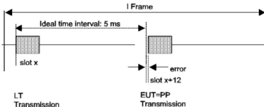
Figure 33: PP packet transmission error definition
