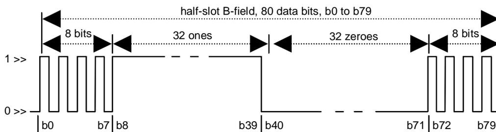
NOTE: Bits  $b_0$  to  $b_7$  and  $b_{72}$  to  $b_{79}$  are alternating 1s and 0s with the even order bits ( $b_0, b_2, b_4, \dots$ ) set to "1" and the odd-order bits ( $b_1, b_3, b_5, \dots$ ) set to "0".
