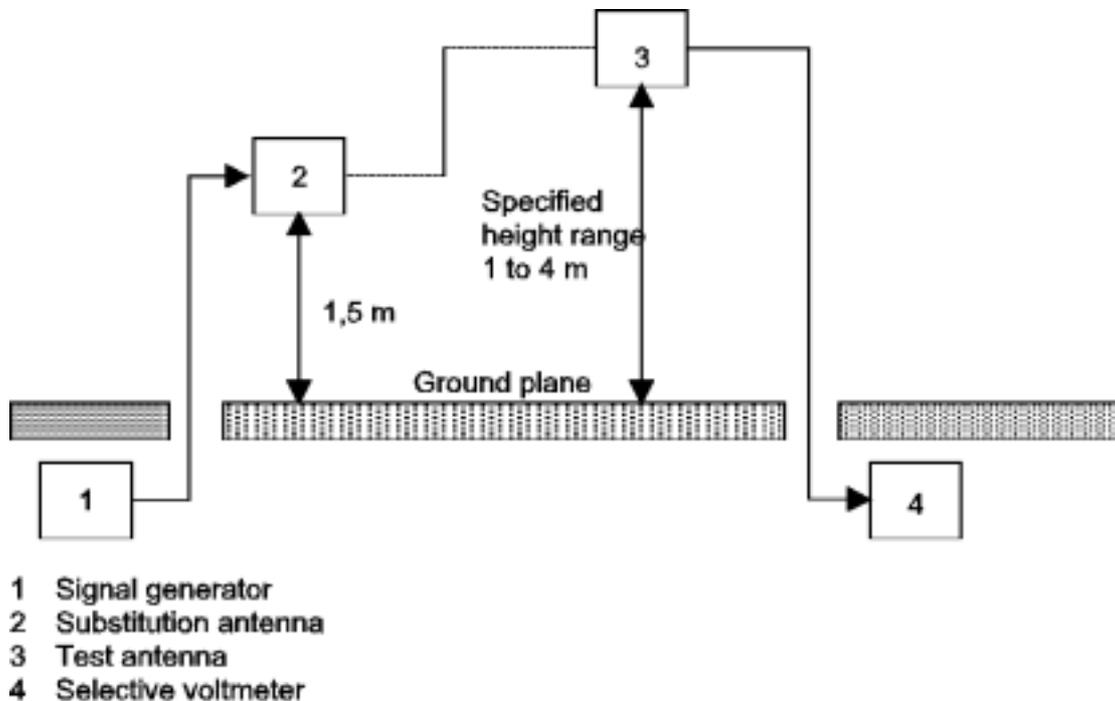
**Figure 11: Measuring arrangement for calibration**
