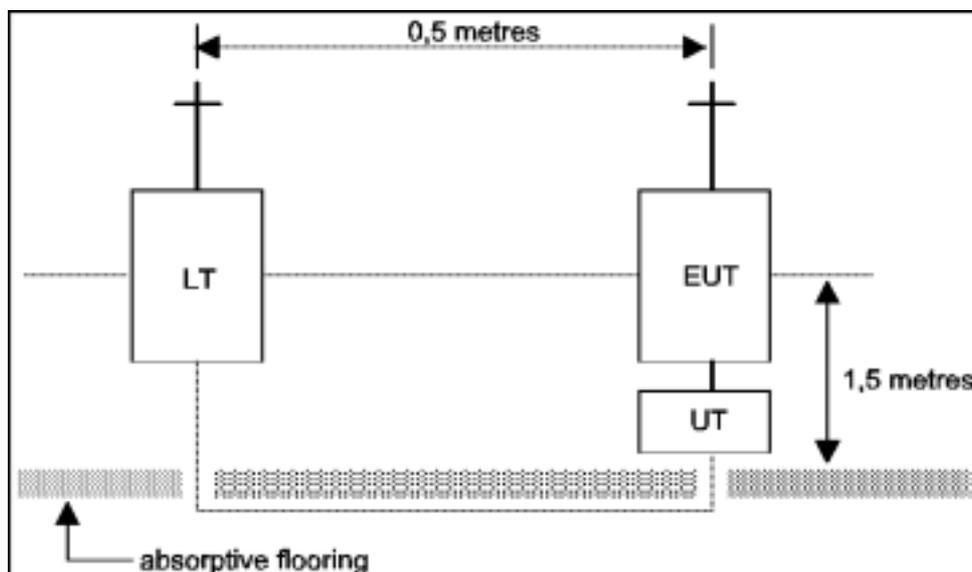
Figure 23: Testing arrangement
