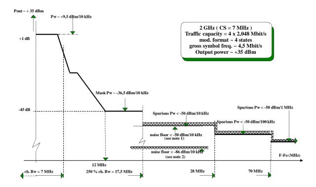
NOTE 1: Typical noise floor with 3<sup>rd</sup> order i.m.p. > 50 dB. NOTE 2: Typical noise floor with maximum input level (highest dynamic range).
