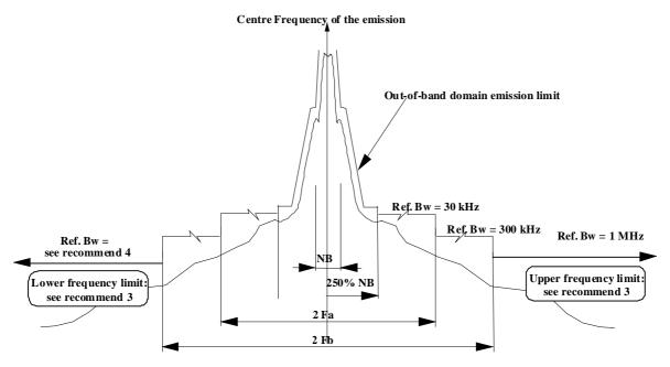
Figure A.2: Generic spurious domain emission reference bandwidth limits mask (ref. to table A.4) for BWA systems operating between 1 GHz and 6 GHz.
