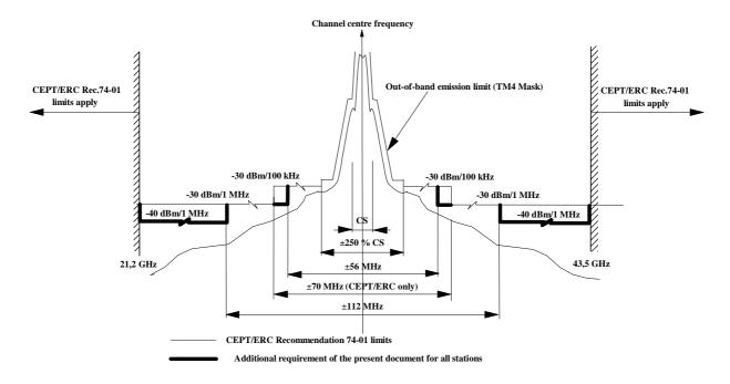
Figure 2: MP equipment for channel separation 1 < CS ≤ 10 MHz
