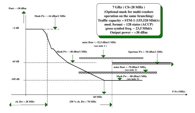
NOTE 1: Typical noise floor with 3<sup>rd</sup> order i.m.p. > 50 dB. NOTE 2: Typical noise floor with maximum input level (highest dynamic range).
