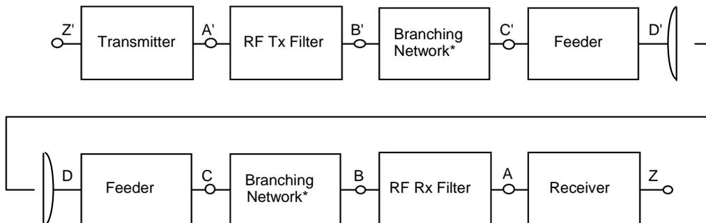
NOTE 1: For the purpose of defining the measurement points, the branching network does not include a hybrid.
