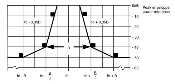
fc = Transmitter carrier frequency
