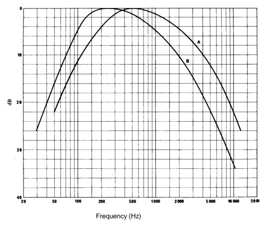
Curve A = Frequency spectrum of standardized noise (measured with one-third octave filters). Curve B = Frequency response characteristics of filter circuit.
