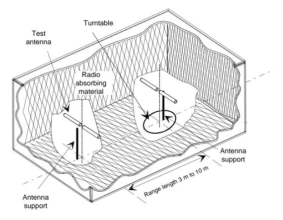
Figure C.1: A typical anechoic chamber
