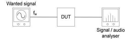
Figure 5: Measurement setup for Rx sensitivity
