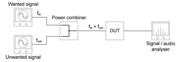
Figure 6: Measurement setup for receiver adjacent channel selectivity
