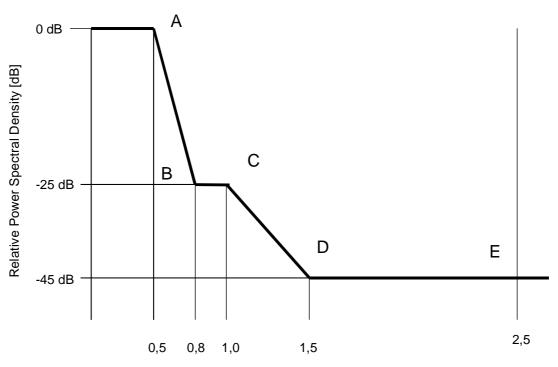
Figure 4: Frequency Hopping Code Division Multiple Access (FH-CDMA) spectrum mask normalized for channel spacing
